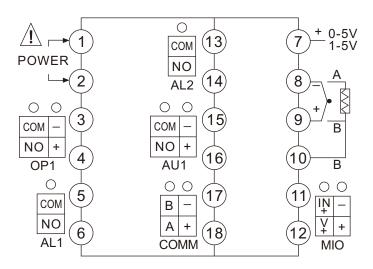
Note: Linear voltage ranges below 1V are input from terminals 8(-) and 9(+), while signals from 0 to 5V and 1 to 5V are input from terminals 7(+) and 8(-); 4-20mA linear current input can be external Connect a 250 ohm high precision resistor to convert it into a 1-5V voltage signal, and input it from terminals 7(+) and 8(-). You can also install I3 and I4 modules on the MIO port to input from terminals 11 and 12(+).
