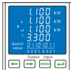
Channel 4, 2 and 1 are closed; Channel 3 is cut off.
