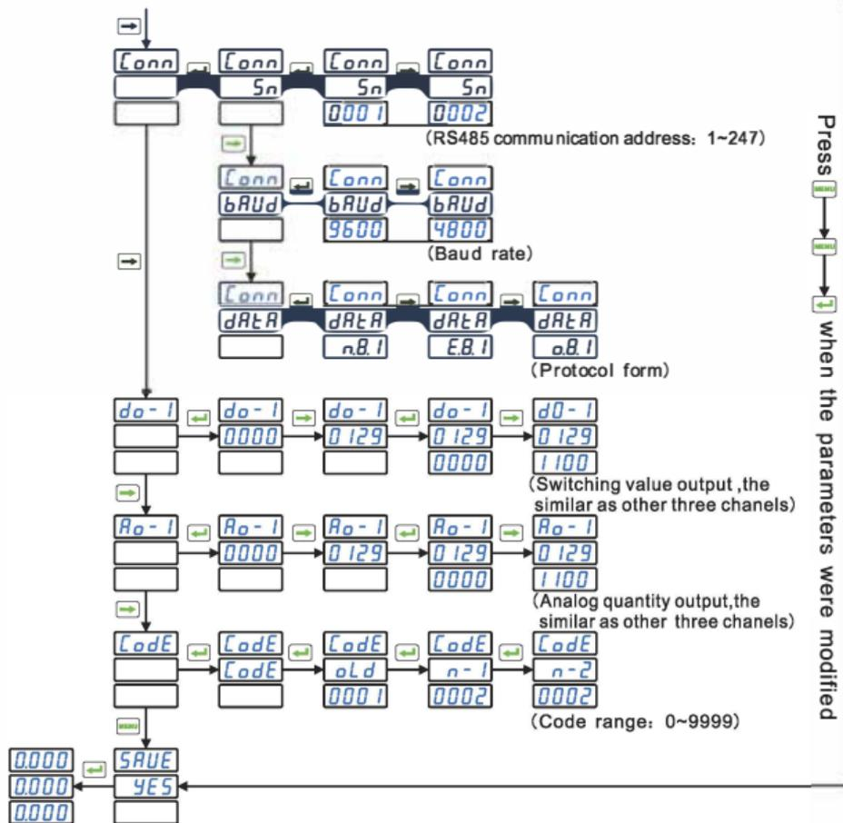
Note:Quit the programming mode, when the instrument displays"save yes", press [right arrow] to save and quit the programming mode.It can not be saved if press [left arrow] button
