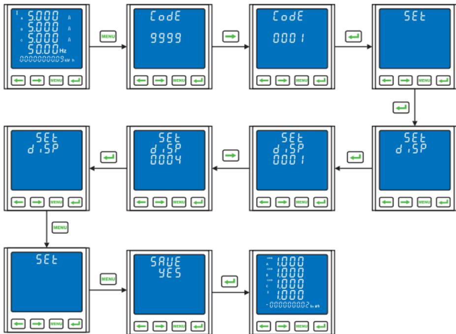
4.6.2 Set signal input net, change the net from n.3.4(3P4W) to n.3.3(3P3W), set multiplying power of current transformer is 60(CT 300A/5A)
