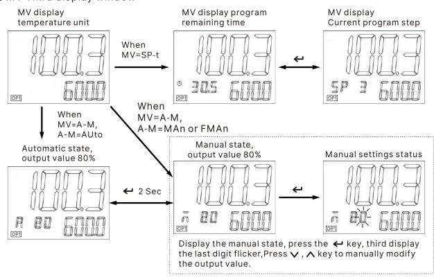
When A-M=FMAn, For manual state only, no manual / automatic state switch.
