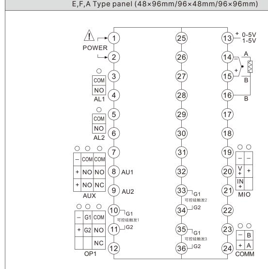
Note: Linear voltage ranges below 1V are input from terminals 14(-) and 15(+), while signals from 0 to 5V and 1 to 5V are input from terminals 13(+) and 14(-); 4-20mA linear current input can be external Connect a 250 ohm high precision resistor to convert it into a 1-5V voltage signal, and input it from terminals 13(+) and 14(-). You can also install I3 and I4 modules on the MIO port to input from terminals 20(+) and 21.
