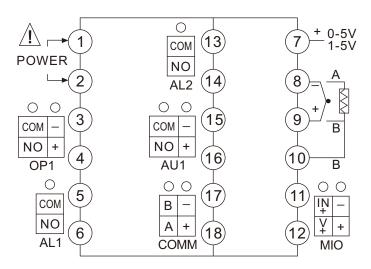
Note: Linear voltage ranges below 1V are input from terminals 8(-) and 9(+), while signals from 0 to 5V and 1 to 5V are input from terminals 7(+) and 8(-); 4-20mA linear current input can be external Connect a 250 ohm high precision resistor to convert it into a 1-5V voltage signal, and input it from terminals 7(+) and 8(-). You can also install I3 and I4 modules on the MIO port to input from terminals 11 and 12(+).
