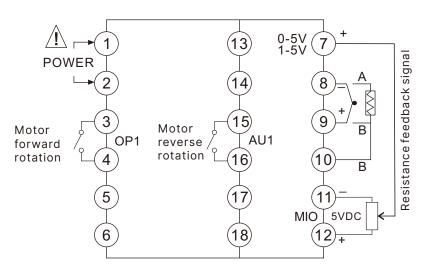
When the valve position feedback signal is a potentiometer, install a non-isolated 5V power distribution output module V5 to convert the resistance signal into a voltage signal (as the picture shows).
