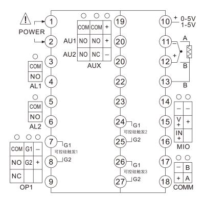
Note: Linear voltage ranges below 1V are input from terminals 11(-) and 12(+), while signals from 0 to 5V and 1 to 5V are input from terminals 10(+) and 11(-); 4-20mA linear current input can be external Connect a 250 ohm high precision resistor to convert it into a 1-5V voltage signal, and input it from terminals 10(+) and 11(-). You can also install I3 and I4 modules on the MIO port to input from terminals 15(+) and 16.
