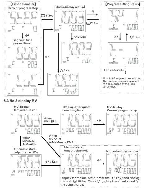
When A-M=FMAn, For manual state only, no manual / automatic state switch.
