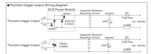
Note 1: According to the voltage and current of load, choose suitable varistor to protect the thyristor. Capacitor resistor absorber is needed for inductance load or phase-shift trigger output.
