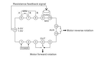
When the valve position feedback signal is a potentiometer, install a non-isolated 5V power distribution output module U5 to convert the resistance signal into a voltage signal (as the picture shows).
