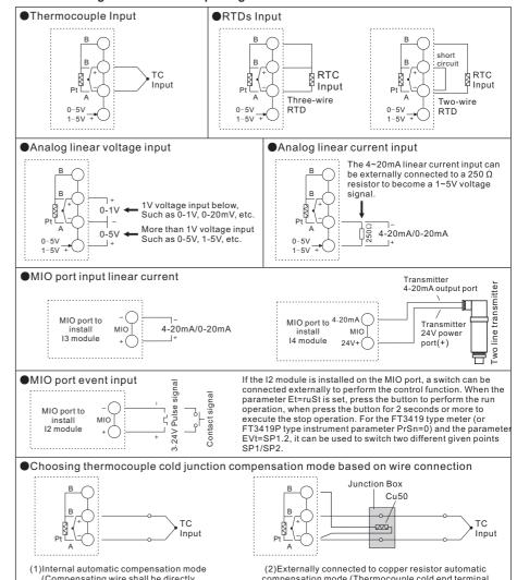
(Compensating wire shall be directly connected to the connection terminals) compensation mode (Thermocouple cold end terminal box had better keep away from heat sources)
