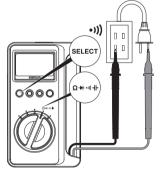
The buzzer beeps at 10 to 50  $\Omega$  or less.
