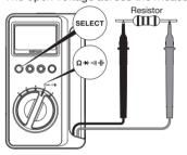
If measurement is likely to be influenced by noise, shield the object to measure with negative potential (COM). If a finger touches a test pin during measurement, measurement will be influenced by the resistance in the human body, and that results in measurement error.
