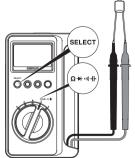
Discharge the capacitor before It takes a while to measure large
