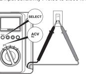
Set the function switch to ACV. Each press of the SELECT button alternates ACV and Hz. appears on the display when a voltage of 20 V or more is input. At the moment the input exceeds 20 V. the buzzer beeps and the backlight flashes to indicate it.
