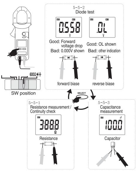
Each time the SELECT button is pressed, the functions change as indicated by  $\rightarrow$  in the figure.
