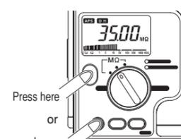
Press the **MEASURE** or **LOCK** button to stop outputting the test voltage.
