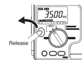
Release the **MEASURE** button to stop outputting the test voltage.
