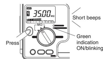
The test voltage is output when the **MEASURE** button is held pressed. **F** appears and short buzzer sounds during this operation.
