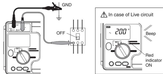
⚠ If the object to be measured is a live circuit ( $\geq 30$  V AC/DC), the voltage is displayed, buzzer sounds, and the ALARM indicator lights up. In this case, the test voltage cannot be output by pressing the MEASURE or LOCK button. Disconnect the power supply from the object to be measured and try again.
