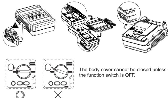
The body cover cannot be closed unless the function switch is OFF.
