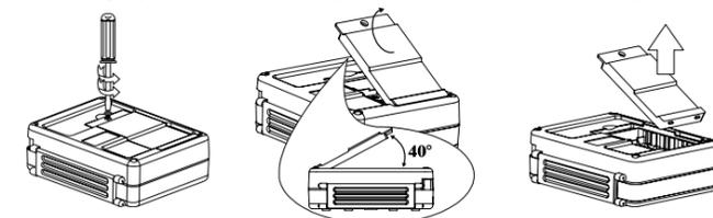
Note: Use caution with battery polarity when replacing batteries.
