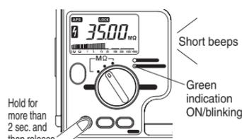
Press and hold the **LOCK** button for more than 2 seconds to output the test voltage continuously. **F** and **LOCK** appears and short buzzer sounds during this operation.
