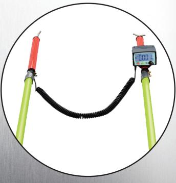
MDP-50K must be connected with an approved hot stick, such as HS-175, HS-120, HS-120R to do the high voltage measurement.
