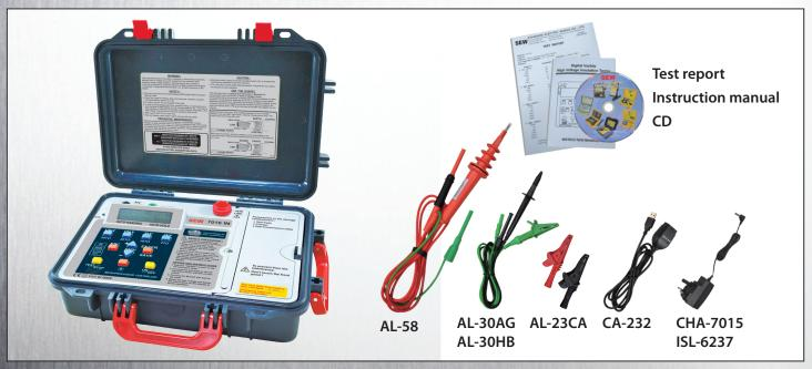
A complete set of accessories : H.V test leads (AL-30AG AL-30HB), Alligator clip (AL-23CA). H.V Line probe with (AL-58), Data transmission cable (CA-232), Charger (CHA-7015), Compact disk(CD), Instruction manual, Test report.
