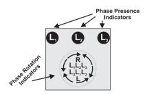
3 Phase sequence Rotation indicator circuit: This circuit has also a LCD indication This product does not require any battery as it takes its power from the circuit under test.
